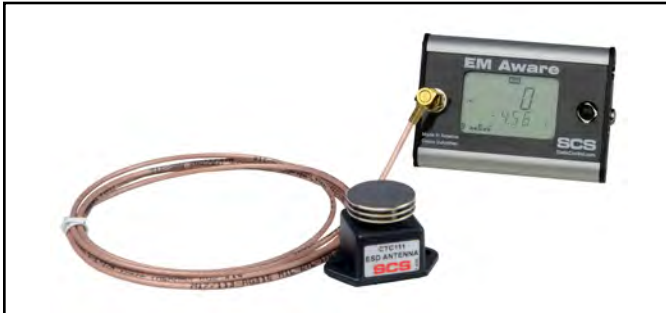
Figure 1. SCS 770066 EM Aware Monitor with standard antenna
