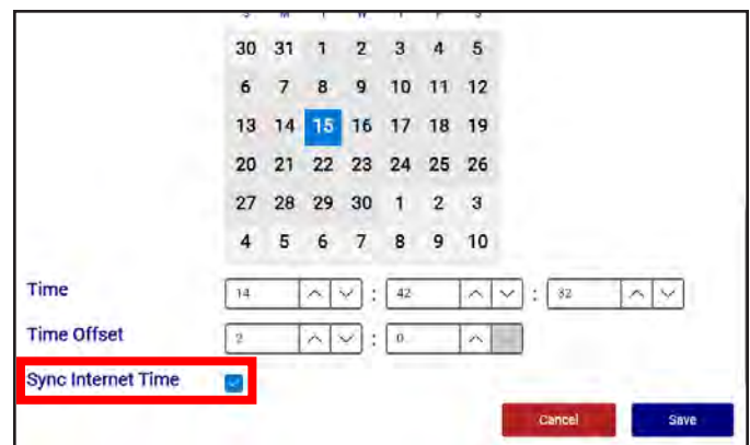
Figure 18. Enabling the Sync Internet Time feature
