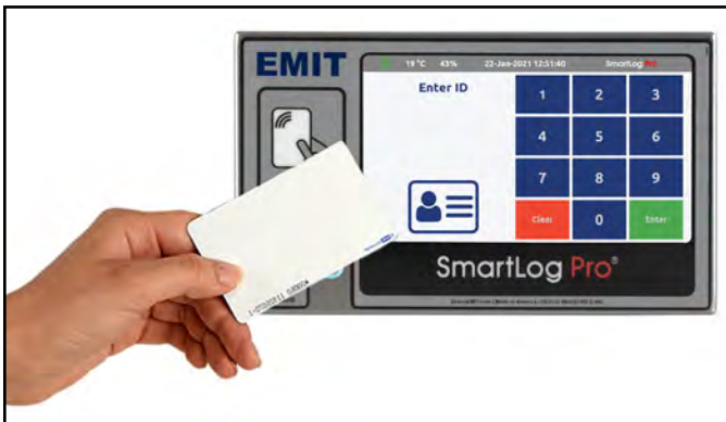
Figure 23. Holding a proximity badge in front of the RFID icon on the SmartLog Pro® 2
