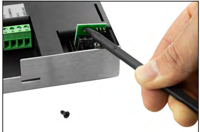
Figure 28. Lifting the used dual-wire wrist strap jack from the SmartLog
