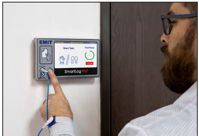
Figure 24. Performing a single-wire wrist strap test
