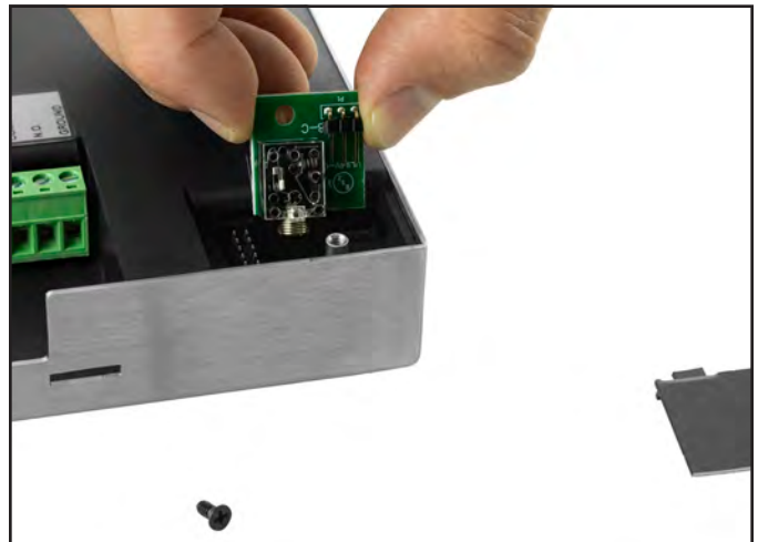
Figure 29. Installing the replacement dual-wire wrist strap jack
