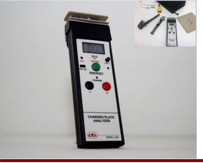
Validate the performance of your static control system. Apply a calibrated charge to objects, surfaces, or static fields and accurately measure the time for discharge to a 10% cutoff. Measures static field strength.
