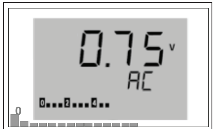
Figure 9. AC voltage display
