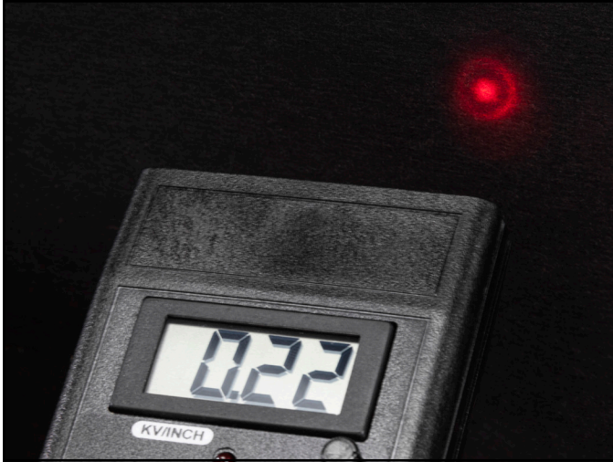
Figure 7. Aligning the two bullseyes emitted by the LED range indicator
