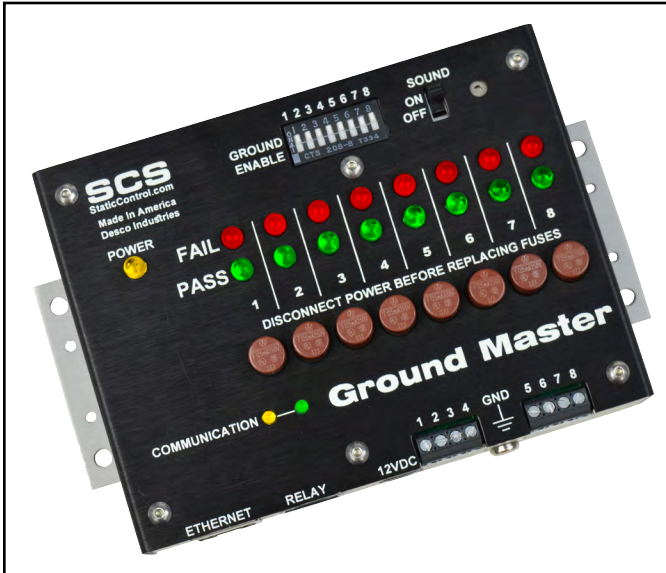
Figure 1. SCS 770060 Ground Master Monitor
