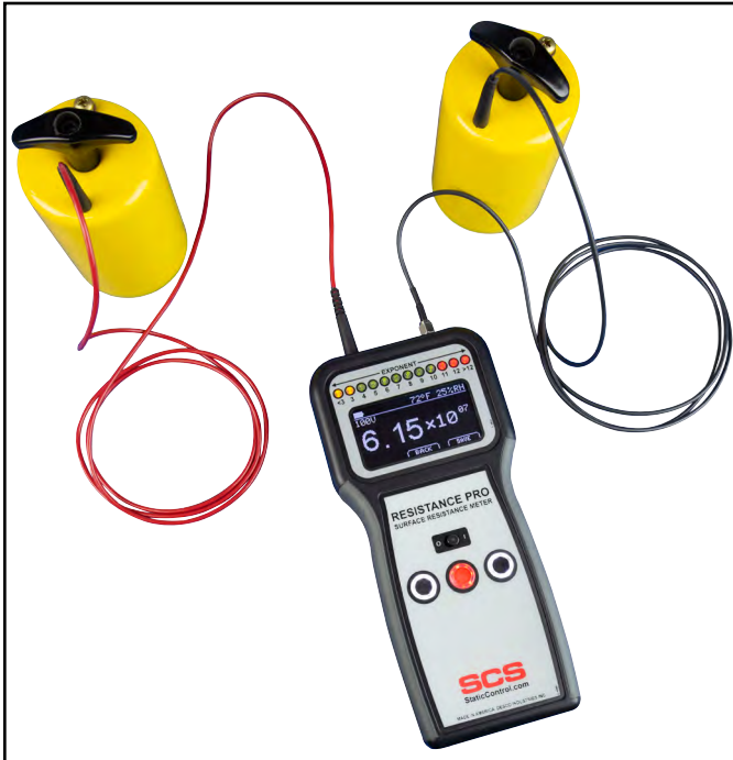
Figure 1. SCS Resistance Pro Meter Kit
