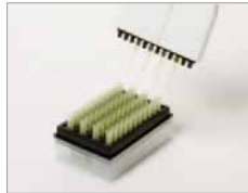
3. Turn the rack and use the multichannel pipette (skipping every other row) and install the tips in the remaining row.
