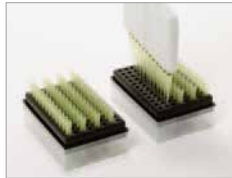
2. Transferring tips using a multichannel pipette, leaving the last row empty.
