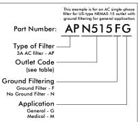
**Outlet** Configuration OUTLET ORDERING CODE OUTLET ORDERING CODE 0 N515 CN1A \$0 ~125V 3A NEMA 5-15 CHINA Ο EUSK EUUK 0 \_ ~250V 3A schuko пк .... TS03 . . . FERMINAL BLOCK SINGLE PHASE 3A
