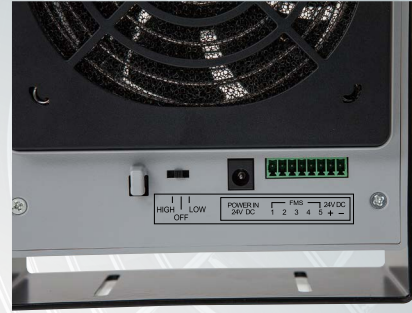
Facility Monitoring System Interface
